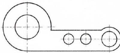
11. Copy the sketch to 1:1 scale and dimension it using unidirectional system with Chain dimensioning method
